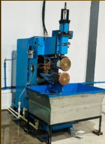
Seam Welding machine 100KVA
